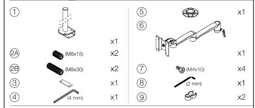
1 Position and mount the clamp 1 to the table. For tables thinner than 21 mm, use screws (28). Position the metal sheet 3 and fasten it using the 3 Once the pole is screws and Allen key(4) (See illustration). fastened, insert the cosmetic plastic cover(5) into the pole and ascertain its position.
